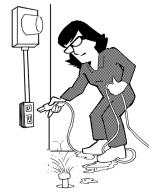
**Electrical safety:** Maintain cords in good condition. Use ground-fault-circuit interrupter (GFCI) cords for outlets in wet conditions.
