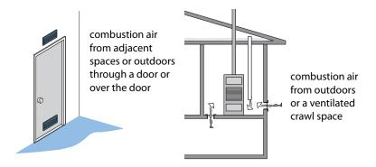
**Passive combustion air options:** Combustion air can be supplied from adjacent indoor spaces or from outdoors. Beware of passive combustion air vents into the attic that could depressurize the combustion zone or allow moist indoor air to travel into the attic. Also beware of taking combustion air from wet crawl spaces.
