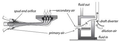
**Atmospheric, open combustion gas burners:** Combustion air comes from the indoors in open combustion appliances. These burners use the heat of the flame to pull combustion air into the burner. Dilution air, entering at the draft diverter, prevents overfire draft from becoming excessive.
