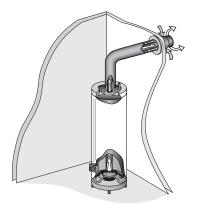
**Direct-vent water heater:** Moves combustion air and flue gases through a concentric pipe system without a draft fan.
