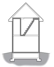
**Insulating and sealing attic stair** walls, doors, and stairs: Insulating and air sealing these is one way of establishing the thermal boundary.
