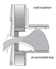
**Balloon framing:** Floor cavities are usually connected to wall cavities. Blow a plug of insulation into the floor cavity to seal this leaky uninsulated area.
