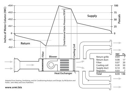
**Visualizing TESP:** The blower creates a suction at its inlet and a positive pressure at its outlet. As the distance between the measurement and blower increase, pressure decreases because of the system's lower resistance.
