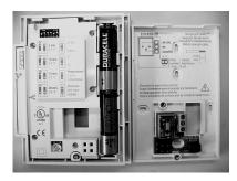
Many models of programmable thermostats have settings that you select from inside the thermostat. These settings include the heat-anticipator setting, which adjusts the cycle length of the heating or cooling system.
