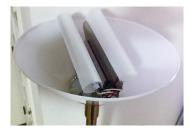
**LED lamps:** These advanced lamps use about one-third of the electricity of the incandescent lamps they usually replace, and they last about ten times as long.
