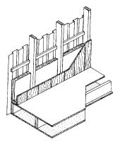
Standard mobile home construction: 2-by-4 walls and 2-by-6 floor joists are the most common construction details.
