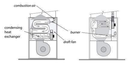
**90+ Gas furnace:** A 90+ furnace has a condensing heat exchanger and a stronger draft fan for pulling combustion gases through its more restrictive heat exchanger and establishing a strong positive draft.
