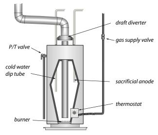
**Standard gas water heater:** These open combustion appliances are often troubled by spillage and backdrafting.
