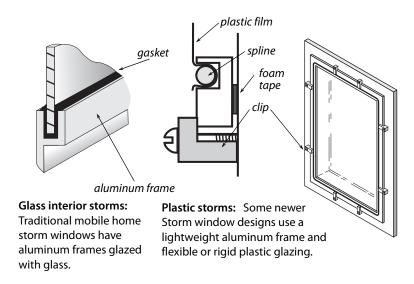
Interior storm windows are common in mobile homes. These stationary interior storms serve awning and jalousie windows. Sliding interior storm windows pair with exterior sliding prime windows.
