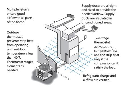
Coil is cleaned every year. Weeds, grass and shrubs shouldn't grow within 3 feet. Verify that no airflow restrictions exist above the outdoor unit.
