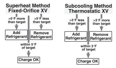
**Charge-checking:** Two methods help technicians judge whether the charge is correct. The remedy for incorrect charge is to either add or remove refrigerant.
