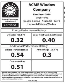
**Example NFRC label:** The key selection criteria for window shopping is displayed on the NFRC label.
