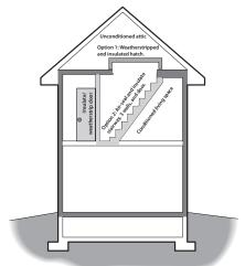
Stairways at the thermal boundary: The stairway may be within the thermal boundary or outside it. Only walls, ceilings, doors, and hatches at the thermal boundary require thorough air sealing. The door as shown is open.
