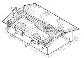
Whole-house fan circulation: the whole-house fan sucks air out of the house and exhausts it into the attic or through a gable wall. Cooler air enters the windows as make-up air for the fan.
