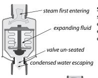
**Steam traps:** Steam enters the steam trap heating its element and expanding the fluid inside. The expanded element plugs the steam's escape with a valve.
