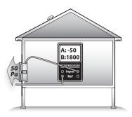
Blower door test: Air barriers are tested during a blower-door test, with the house at a pressure of 50 pascals negative with reference to outdoors. This house has 1800 CFM<sub>50</sub> of air leakage. Further diagnostic tests can help determine where that leakage is coming from.
