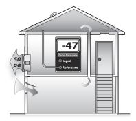
**Zone connectedness:** The attic measures closer to outdoors after the basement window is opened, indicating that the attic and basement are connected by a large bypass.
