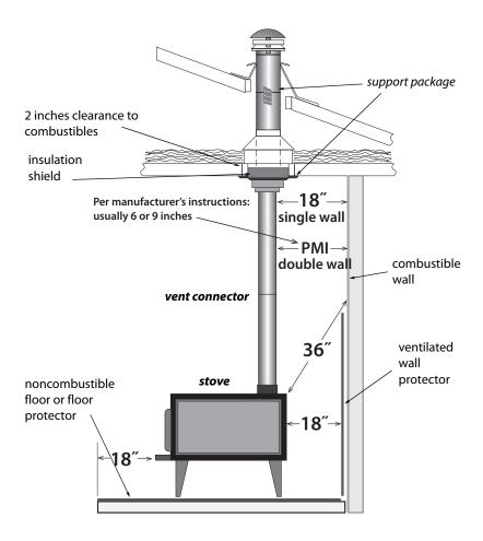
**Wood-stove installation:** Wood-stove venting and clearances are vitally important for wood-burning safety. Read manufacturer's instructions for the stove and its venting components.
