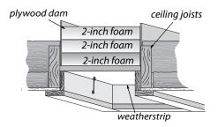
Insulated attic hatch: Building a dam prevents loose-fill insulation from falling down the hatchway. Foam insulation prevents the access hatch from being a thermal weakness. Install foam to achieve atticinsulation R-value of R-49. Foam can be glued together in layers.
