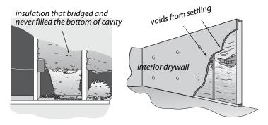
**Problems with low density insulation:** Blowing insulation through one or two small holes usually creates voids inside the wall cavity. This is because insulation won't reliably blow at an adequate density more than about one foot from the nozzle. Use tube-filling methods whenever possible, using a 1.5-inch hose inserted through a 2-inch or larger hole.
