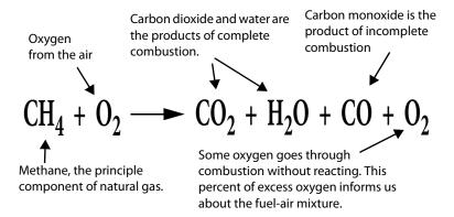
Modern flue-gas analyzers measure  $O_2$ , CO, and flue-gas temperature. Some models also measure draft. Flue-gas analyzers also calculate combustion efficiency or steady-state efficiency (SSE), which are synonymous.
