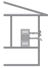
Sealed combustion heaters: Sealed-combustion furnaces prevent the air pollution and house depressurization caused by some open-combustion furnaces.
