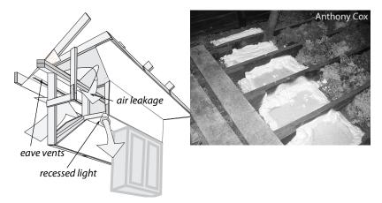
**Kitchen soffits:** The ventilated attic is connected to the soffit and the wall cavity through framing flaws. Any hole in the soffit creates a direct connection between the kitchen and attic. Block off the soffit from the attic with drywall or plywood sealed with two-part spray foam as shown in the photo.
