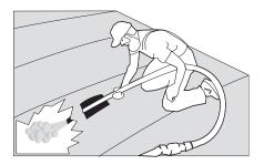
**Roof-top insulation:** Blowing fiberglass insulation through the roof top is effective at achieving good coverage and density on almost any metal roof.
