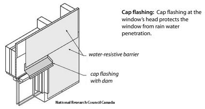
Follow these steps to install a nailing-fin window in the rough opening.
