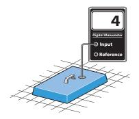
If the ducts are in a basement and the basement is conditioned, pressure pan testing isn't necessary, although air sealing the return ducts for safety is still important.
