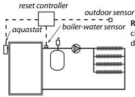
**Reset controller:** This control adjusts circulating-water temperature depending on the outdoor temperature.
