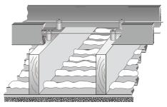
Shielding knob and tube: If you can't decommission knob-and-tube wiring, you may construct a dam to shield it from being covered by insulation.
