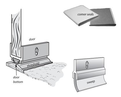
**Weatherstripping at the door bottom:** A threshold and door bottom are the ideal bottom seal for a door. The threshold and door bottom must be adjusted to seal but not bind. Corner seals in the bottom complete a quality doorweatherstripping job.
