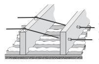
**Knob and tube wiring:** Obsolete and worn wiring should be replaced during energy retrofit work so that building cavities can be sufficiently insulated.
