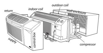
Unitary heat pumps: These unitary ductless heat pumps sit inside an exterior wall. They are a very efficient kind of electric heating and cooling.
