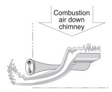
Take all necessary steps to reduce CAZ depressurization and minimize combustion spillage, based on your tests and add make-up air if necessary.
