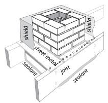
Sealing around chimneys: Chimneys require both an air seal and a shield with a 3-inch clearance above the chimney if retrofit insulation is installed
