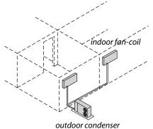
**Ductless mini-split heat pumps:** These systems have very high efficiency: 200% to 400%.
