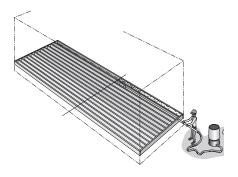
Blowing lengthwise cavities: Floors with lengthwise joists can rarely be filled completely from the ends because of the long tubing needed. The middle can be filled from underneath.
