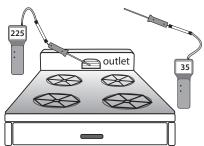
CO from range and oven: Measure CO at oven in undiluted flue gases. Measure ambient CO in the area of the range, but not directly above the burners or oven vent.
