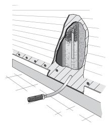
**Tube-filling walls:** This method can be accomplished from inside or outside the home. It is the preferred wall insulation method because it is a reliable way to achieve a uniform coverage and density.
