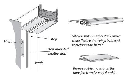
**Weatherstripping doors:** The three weatherstrips shown should be flexible enough to move with the door seasonally and maintain their seal as the door moves seasonally.
