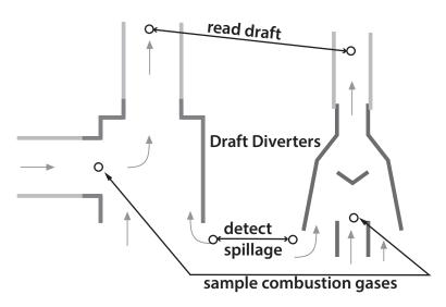
**Testing locations:** This illustration shows two draft diverters and the locations (circles) for draft testing, spillage detection, and sampling of combustion gases.
