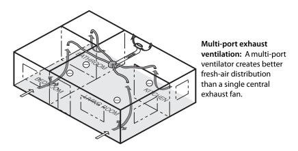
Exhaust ventilation systems create a negative house pressure, drawing outdoor air in through leaks in the shell. This keeps moist indoor air from traveling through building cavities, which would occur with a positive building pressure. The negative building pressure reduces the likelihood of moisture accumula-
