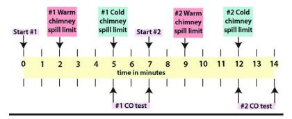
ANSI BSR/BPI - 1200-S-201x Combustion Testing Procedure
