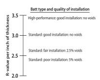
Installers must cut and fit batts very carefully. Batts achieve their advertised R-value only when they are touching all six sides of the cavity it inhabits.
