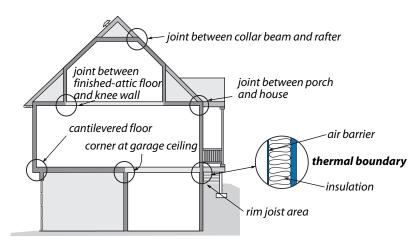
**Air leaks at the thermal boundary:** The air barrier and insulation, which should be adjacent to one other, are located at the thermal boundary. The insulation and the air barrier are often discontinuous at corners and transitions.
