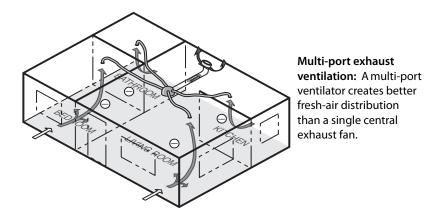
Exhaust ventilation systems create a negative house pressure, drawing outdoor air in through leaks in the shell. This keeps moist indoor air from traveling through building cavities, which would occur with a positive house pressure. The negative house pressure reduces the likelihood of moisture accumulation in building cavities during the winter months in cold climates.
