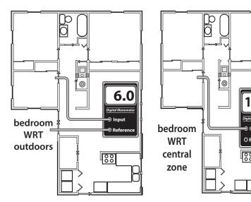
Pressurized bedrooms: Bedrooms with supply registers but no return register are pressurized when the air handler is on and the doors are closed. Pressures this high can double or triple air leakage through the building shell.
