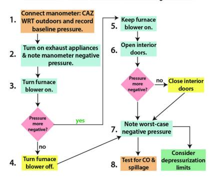
Spillage limits: 2 minutes warm chimney; 5 minutes cold chimney CO limits (ppm): 400 AF/200 AM for furnaces and boilers 200 AF/100 AM for water heaters and space heaters AF = air free; AM = as measured; ppm = parts per million
