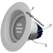
Airtight LED retrofit for can lights: These retrofit fixtures provide a low-wattage LED with a low-air-leakage enclosure that inserts into the existing can light.
